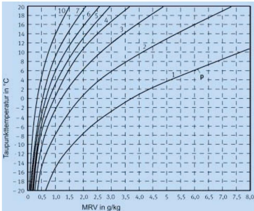
In order to evaluate the absolute humidity content (e.g. MRV) of air, it is therefore often advantageous to measure the dew point in the compressed gas (at higher pressure). Because of the measuring principle of the capacitive polymer sensors used here, exact measured values can be achieved same as measurement in expanded air.
