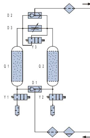
The dryer consists of two drying columns (Q1 and Q2), which alternatively goes into operation or regeneration mode. The cartridge, through which the compressed air passes, dries it and absorbs the water contained in the air. Meanwhile, the second cartridge is flown through in reverse direction by expanded dry air and hence dried out. After some time the two columns are interchanged and the drying process is continued with the column regenerated earlier.
