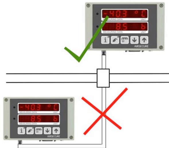
**In order to prevent accumulation of condensation in the case of a fault, the device must be vertically screwed onto the line from above.**
